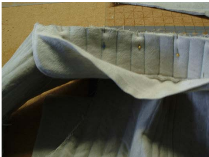
Stitching on the collar keeping the lining free.
